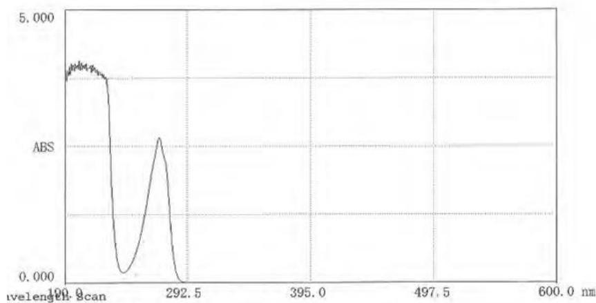
*Fig.2. UV-Spectrum of Phenyl-dextran in water*
