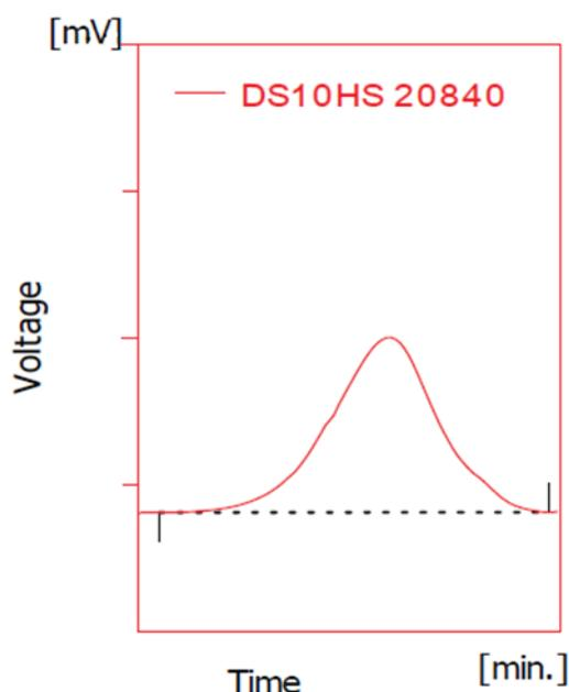
*Figure 2. A typical weight distribution of dextran sulfate 10. The dimensions of dextran sulfate fractions are best described in terms of  $M_w$ ,  $M_n$  and ratio  $M_w/M_n$ . These values are generally determined by gel permeation chromatography which gives information on the molecular weight distribution.*
