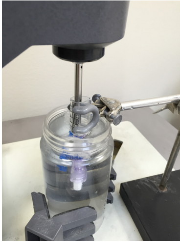
Figure 3 - A 10 ml syringe, which has been cut from the plunger end, clamped to a stand, and placed in an ice water bath.
