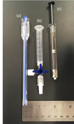
Figure 2 - Homogenizing blade - 0.5 cm diameter (a), Syringe with a 3-way stopcock (b), Hamilton glass syringe - 1 ml (c).
