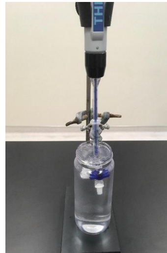
Figure 3 - A syringe sealed with a 3-way stopcock, clamped to a stand, and placed in an ice water bath.
