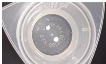
Figure 4 - An intact, stable emulsion on the water's surface
