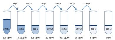
3. **Prepare Samples**: Prepare sample solutions in 1.5 ml centrifuge tubes or disposable culture tubes. If the collagen concentrations of the samples are unknown, preparing multiple samples with varying dilutions using 0.05M acetic acid is recommended.
