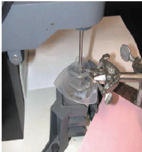
Figure 3 - A 10 ml syringe, which has been cut from the plunger end, clamped to a stand, and placed in an ice water bath.
