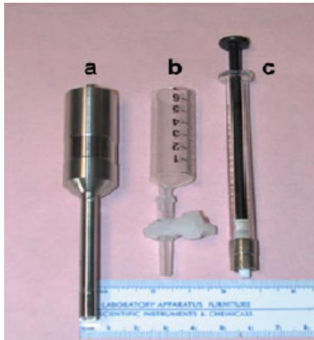
Figure 2 - (a) Homogenizing blade - 0.5 cm diameter (b) Cut syringe - 10 ml with a 3-way stopcock (c) Hamilton glass syringe - 1 ml
